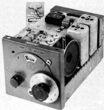
Interior view of modified receiver. Converter is in box with crystal on top.
