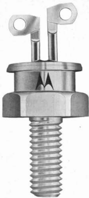
Metal-stud package used for the 8-ampere 200V 2N4170 scr and MAC2-4 triac.
